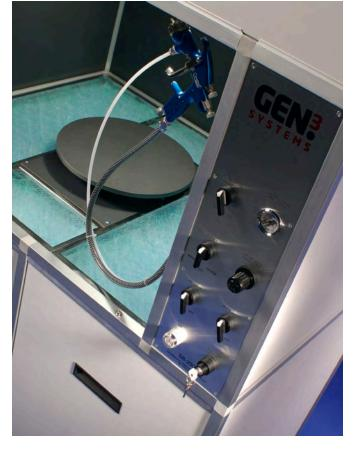
If the semi-automatic foot control for the turntable indexing system is adopted then this is connected to the manifold. The operator passes the spray gun at an angle of 45° over the PCAs which are supported on spigots that are mounted on the turntable.
