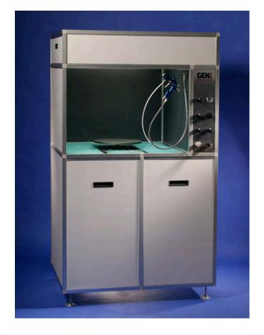
The plenum chamber beneath the turntable is designed to hold the easily removable primary, secondary and tertiary filters and has a 250 mm diameter x 75 mm exhaust spigot.
